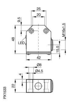
Inductive Sensors BES 516-340-H2-Y 22 x 42 x 48 normally-closed Sn=5mm shielded
